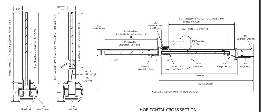
NOTE: Glazing material for all KD units and glazed units must conform to Anzi Z97.1 and CPSC Standard 16 CFC 1201 Category I and II.
